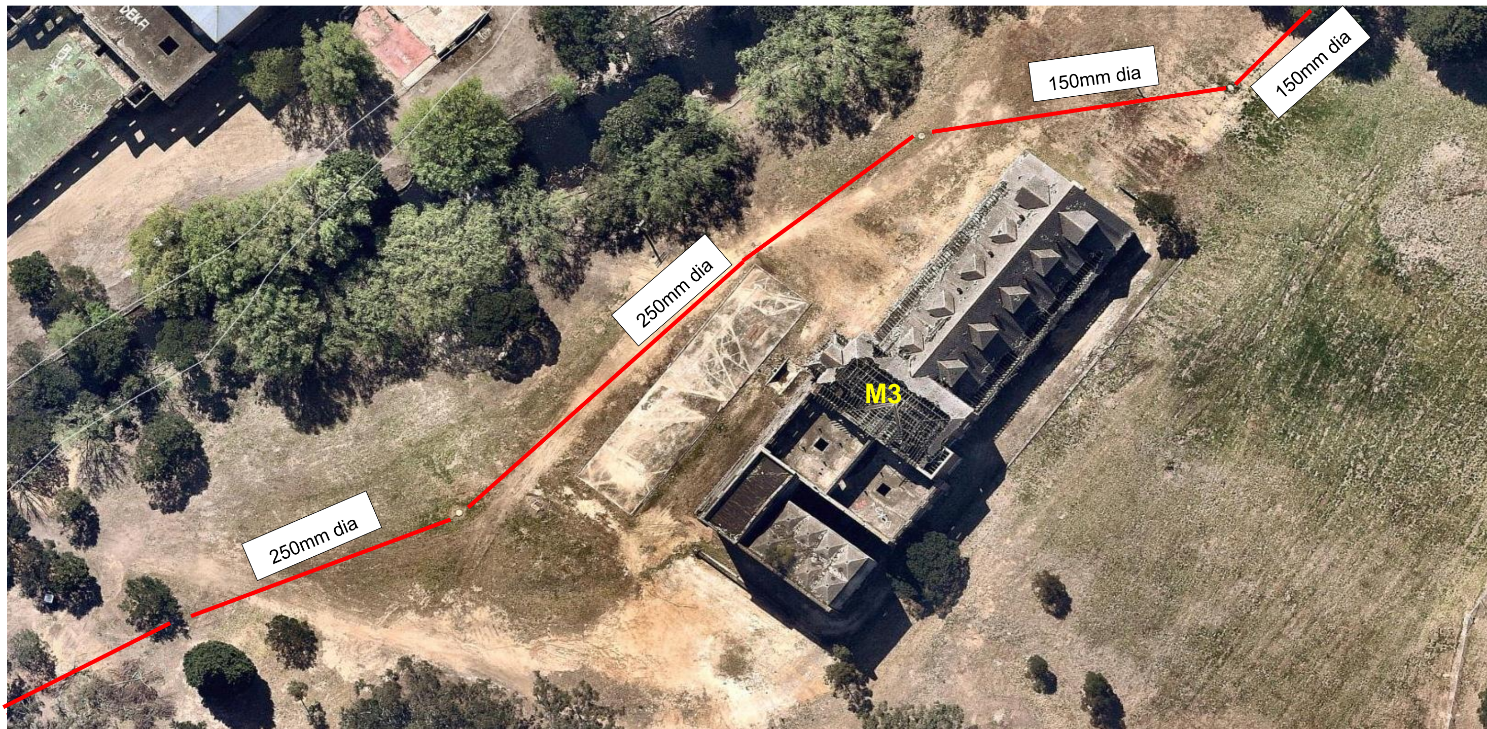
Figure 4 - Existing Sewer Carrier alignment and access pits location beside Maltings 3
